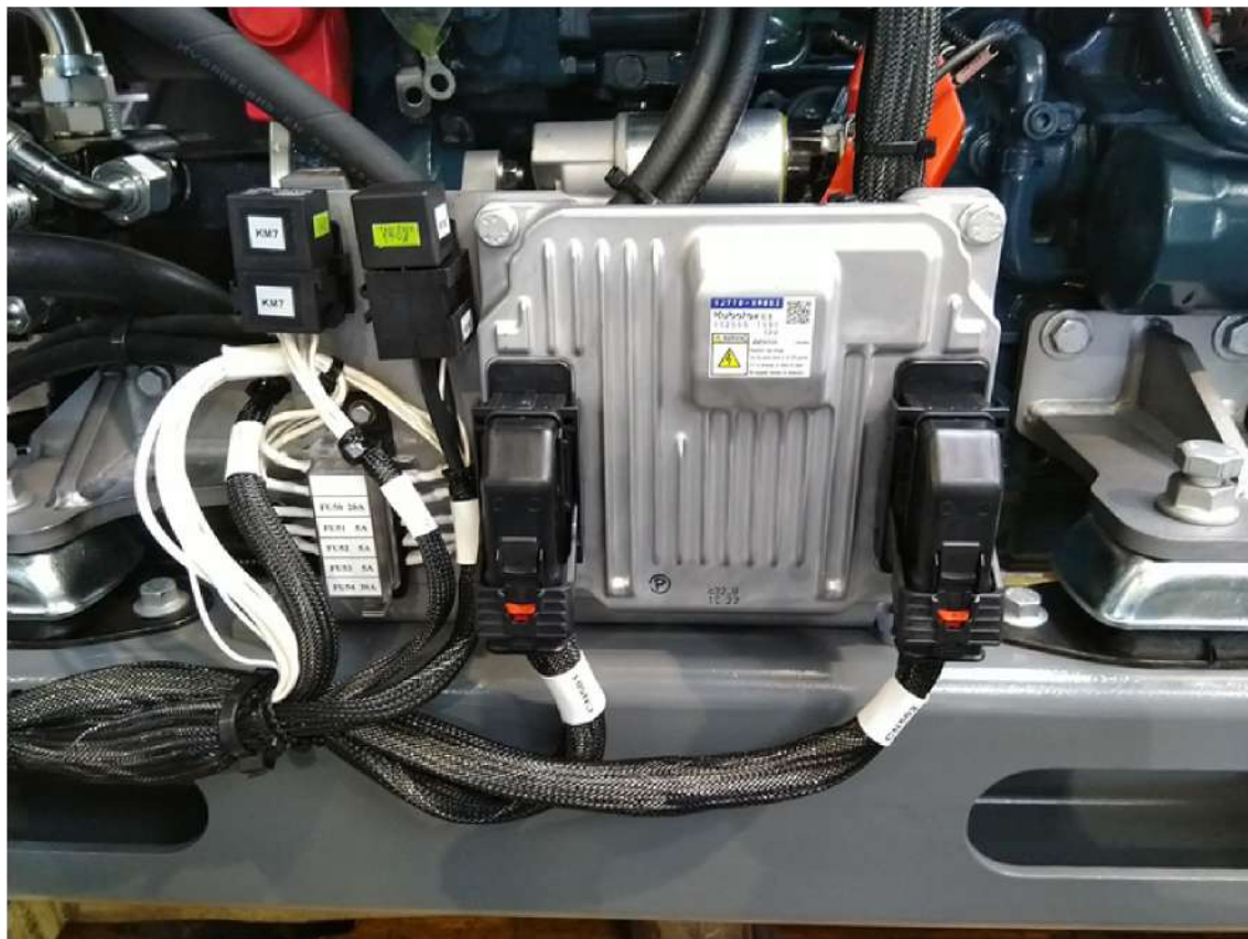
Location of components and EDC module for Kubota engine
